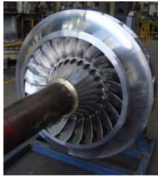
Redesigned martensitic stainless steel runner.
